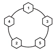
Figure 4-3. Wheel Nut Tightening Sequence
